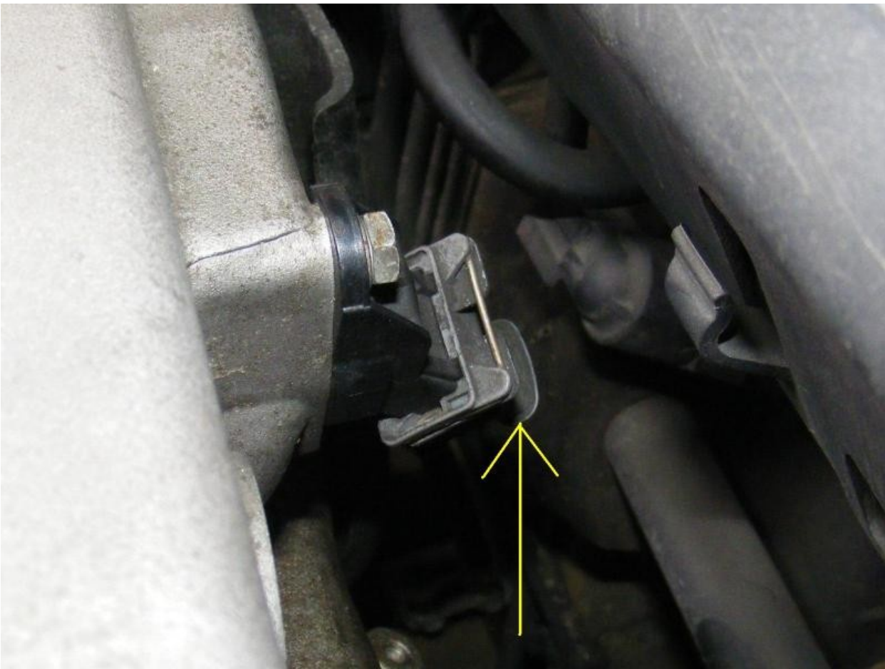
MAP sensor connector is underneath it at the back of the inlet manifold:
